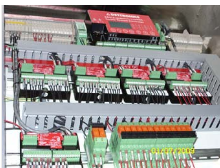
Production of Det-Tronics EQP System designed for Zone 2 Hazardous Area
