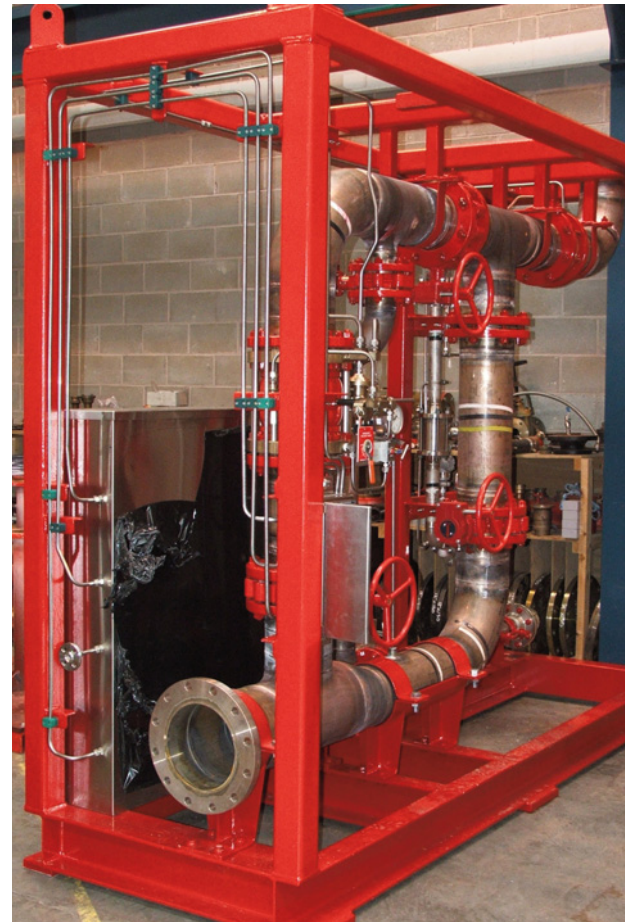
Figure 1. Typical open box frame deluge skid
